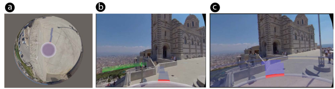
Figure 2: Early prototypes [2]. (a) Blocks representing ROIs were directly embedded in the 360° scene (top-down view). (b) Snap-to-periphery: out-of-view blocks snapped to the periphery. (c) Ring: the ring bands indicated out-of-view blocks.
