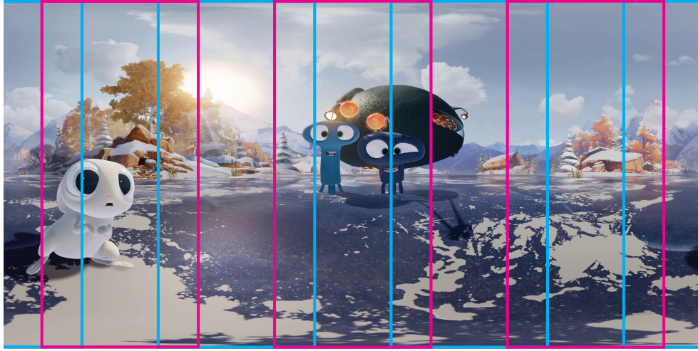
Figure 4.3: Discretized view directions. This figure visualizes the FOVs of |\mathbb{V}| = 6 discretized view directions evenly spaced around the equator on an equirectangular frame from an example video. In our implementation, we used |\mathbb{V}| = 40 . The horizontal FOV of each discretized view matches the horizontal FOV of the Oculus Rift and covers the full vertical range of the video.
