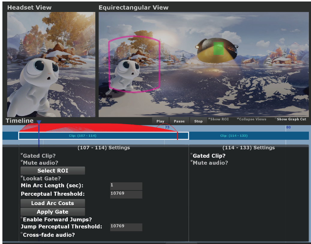
Figure 4.2: Our prototype desktop video editing interface with a gated clip . The upper left pane shows a preview of the headset FOV, which is output live to the Oculus Rift. The upper right pane shows the full equirectangular view and marks the current headset FOV (pink border). The video timeline on the bottom acts as a conventional video editor, with each dark blue rectangle representing a clip. The first clip is a gated clip (white border). Filmmakers specify a gate timecode (red vertical line on timeline), a ROI (green box) on the equirectangular frame, as well as other parameters shown in the settings box below the clip. View-dependent arcs are shown as backward arcs (red arrows) on top of the gated clip. In this example, the ROI is the aliens, and the gate condition is a lookat gate , i.e., playback may not advance past the gate timecode unless the viewer is looking at the ROI. To avoid static loops and reduce arcs with visual artifacts, the filmmaker can set thresholds on the length of arcs and on the perceptual difference of arc transitions. After setting all thresholds, the filmmaker can generate the view-dependent arcs by loading in (pre-processed) arc costs and applying the gate. To have viewers jump to the gate timecode as soon as they see the ROI, the filmmaker can also enable forward arcs that are under a perceptual threshold. Finally, the filmmaker can choose to cross-fade the audio during loop transitions or choose to mute the audio entirely.
